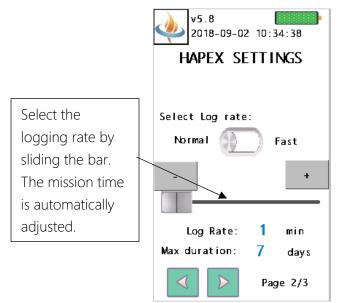
**N.B:** The "fast" mode is a special mode that is useful to do sensor placement testing. In this mode, the sensor will log data every 4 seconds. In this mode though, the internal memory will be full in 6 hours, so it is not very useful for long term deployment.
